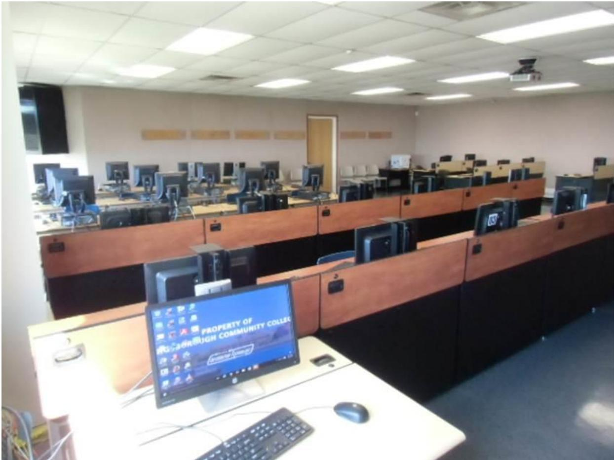
2. Project NO WAIT, 138 Podium and Lab computers were outfitted with SSD cards to reduce the boot time on these computers from 160 seconds to under 55 seconds.
