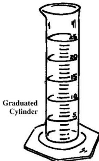
The instructor will explain how to read a graduated cylinder, especially what is meant by the “meniscus” and how to avoid the error of *parallax* in reading the level.
