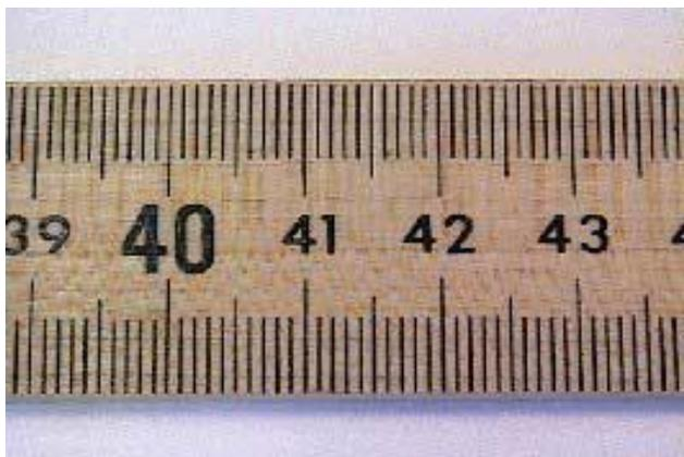
**Figure 1.** This meter stick is calibrated in centimeters (shown as the numbered major divisions) with a smallest number of millimeters.
