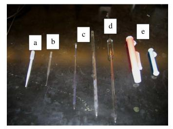
b. Disposable glass Pasteur pipet. These pipets are also used for transferring liquids dropwise.
