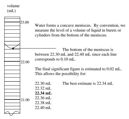
In burets and pipets it is common to measure the volume delivered. This means that two volume measurements will be made. The volume delivered is the difference in these two volumes,  $V_{\text{final}}$  -  $V_{\text{initial}}$
