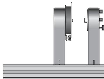
3. Put the rack from the Linear Translator through the slot in the side of the Rotary Motion Sensor. Put the rack clamp onto the rack and tighten its thumbscrew.
